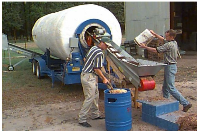
Gambar 6. Rotary Drum Composters
